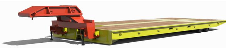
For wider cargo, we developed the Double-wide rolltrailer concept where two 40 feet rolltrailers are placed side by side, and joined together by a coupling system. A twin gooseneck, developed on a Höegh design, ensures the tugmaster has a firm hold of the rolltrailer at all times during transport.
